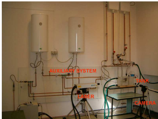
Fig. 2. Auxiliary system, experimental tank with laser and camera
